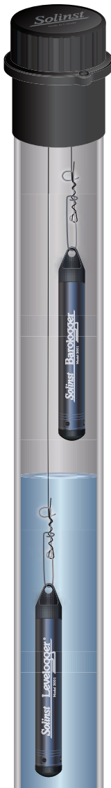
Figure 10-12 Levellogger and Barologger in Well
