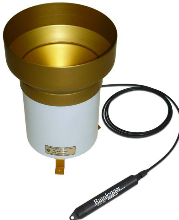
Figure 10-15 Rainlogger Edge Connected to Tipping-bucket
